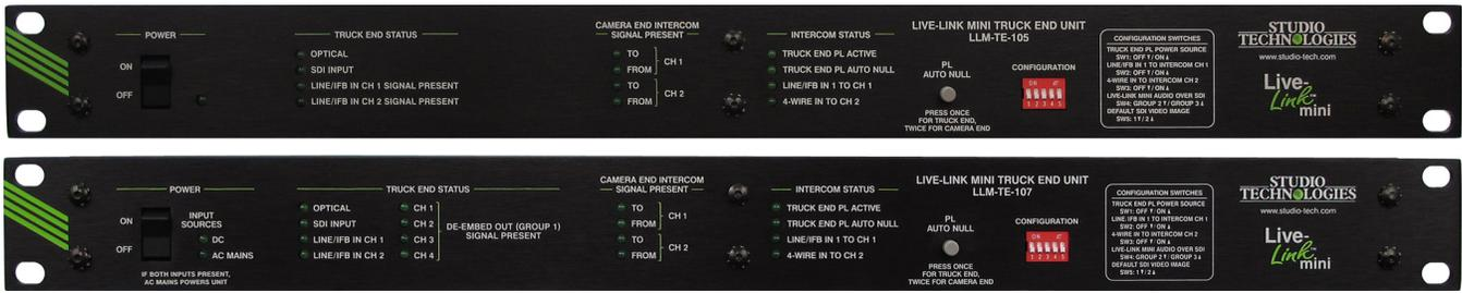
Live-Link Mini Truck End Unit Front Views – Standard Rack-Mount Version (top), Advanced Rack-Mount Version (middle), and Portable Version (right)
